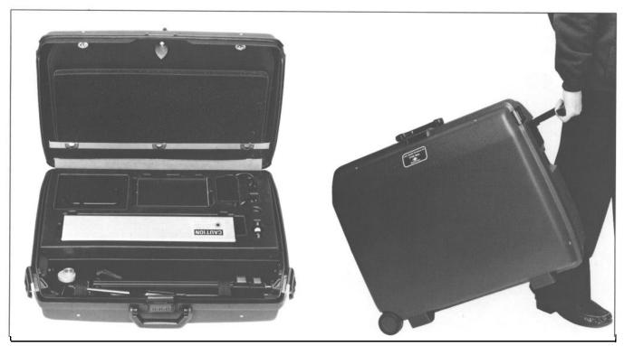
Fig.10. The Type 3544 comes complete with a sturdy carrying case which can contain the Type 8323, the Type 8315 and including the tripod and spare battery box
